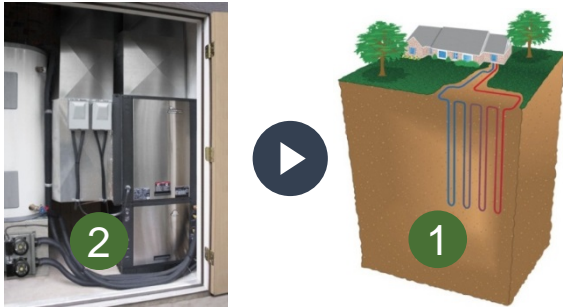
Typical Residential Geothermal System
